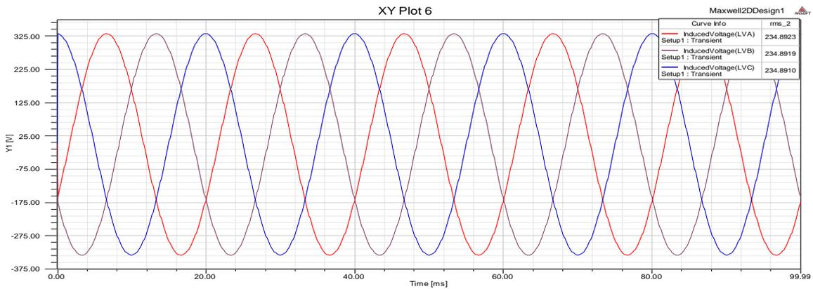
Fig. 9. Induced voltage in low voltage windings
