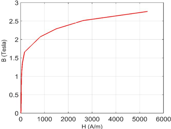
Fig. 2. B-H curve of the transformer [17]
