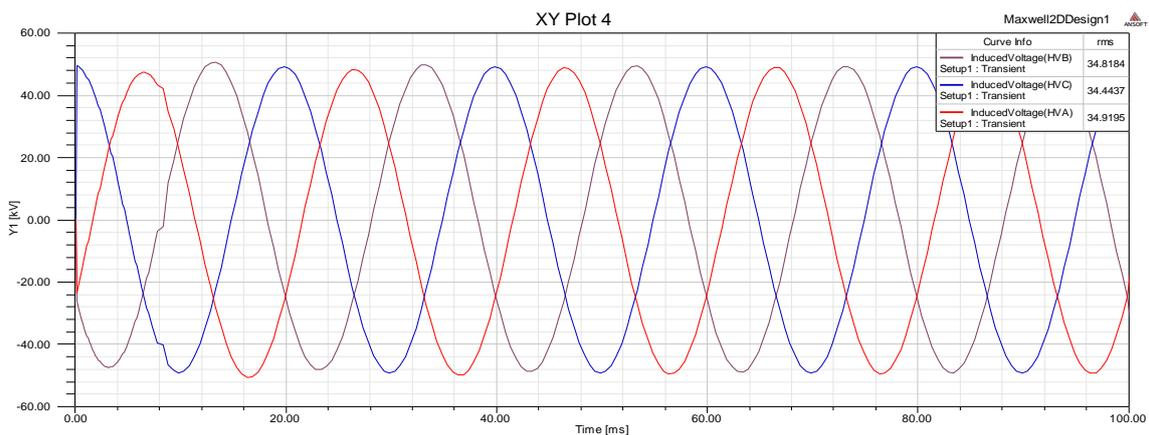
Fig. 10. Induced voltage in high voltage windings
