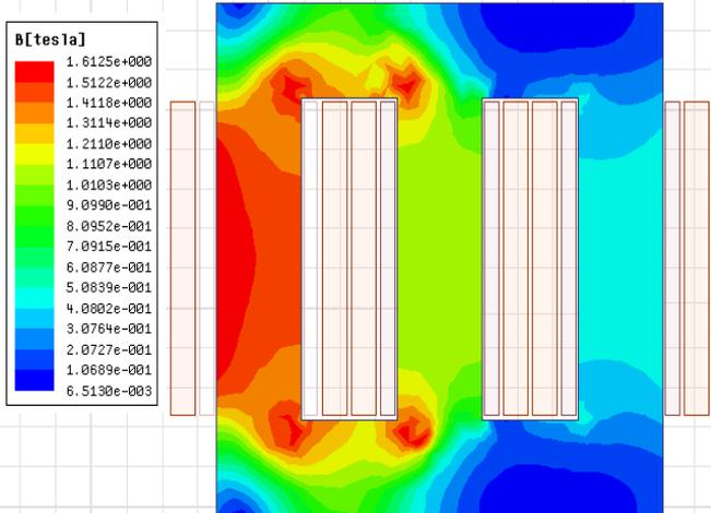
Fig. 12. Magnetic flux density distribution of 2-D full model
