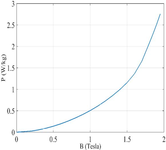
Fig. 3. B-P curve of the transformer [17]
