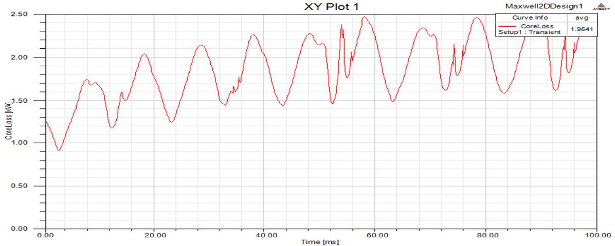
Fig. 16. No-load losses using 2-D half model
