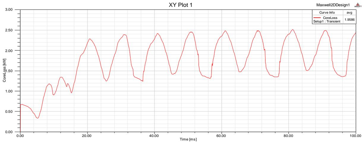
Fig. 15. No-load losses using 2-D full model
