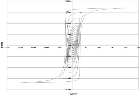
Fig.4. Magnetization curves of the core material [17]
