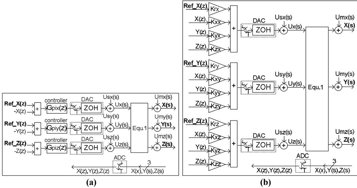
Figure 1. The Lorenz chaos control model with the noise, (a) PI, (b) LQR control model
